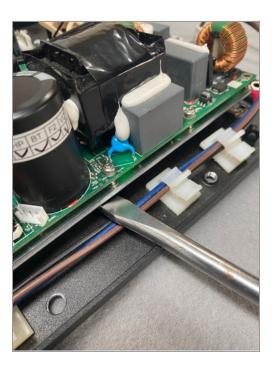
19. Use paper cloth to clean any leftover thermal paste sticking to the bottom plate.
