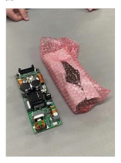
21. Turn the amp over, so the metallic plate faces up. Put three thermal pads onto it. Distribute them evenly, without covering the screw holes.
