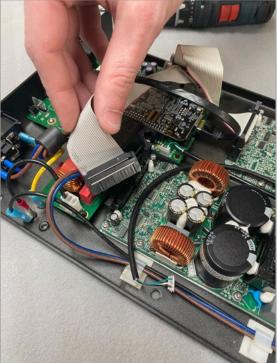
17. Remove the amplifier from the bottom plate. You can put a piece of paper cloth over the thermal paste sticking to the bottom to prevent it from getting on your clothes.
