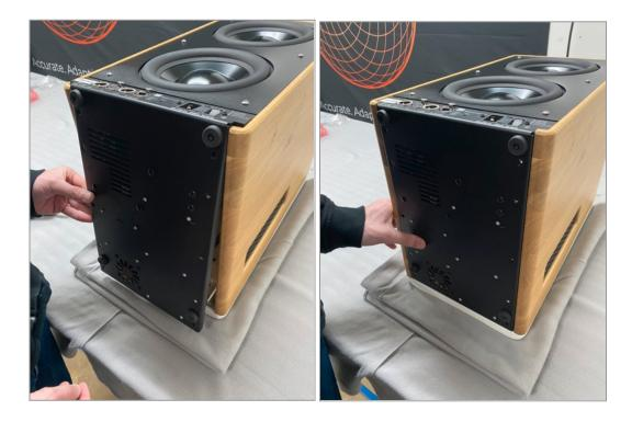
34. Fasten the panel with the 6 Torx screws.
