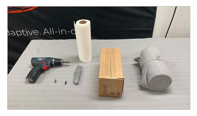
Make sure the automatic screwdriver is put on low resistance (5 or 6) to avoid damaging the screws.
